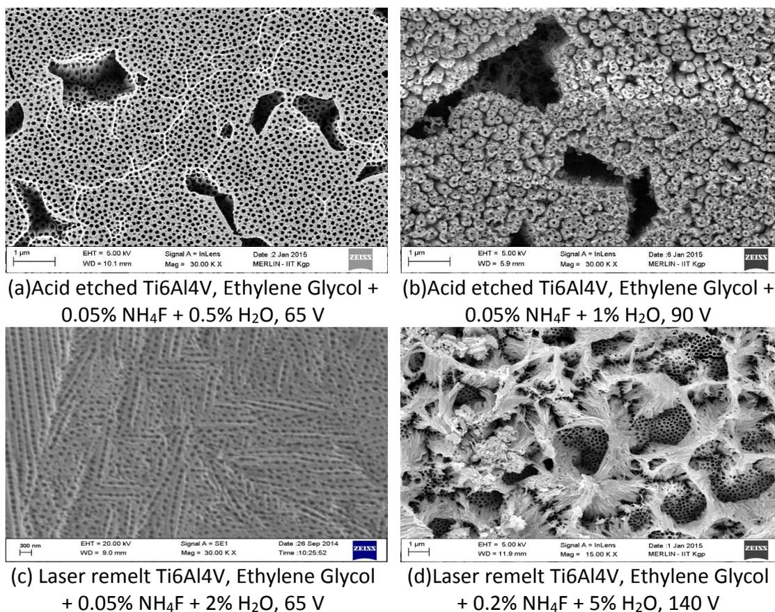
Figure: Surface morphologies after anodization under different experimental conditions.
