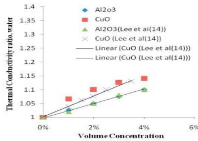
Figure: With the use of nanoparticles: enhancement of thermal conductivity.
