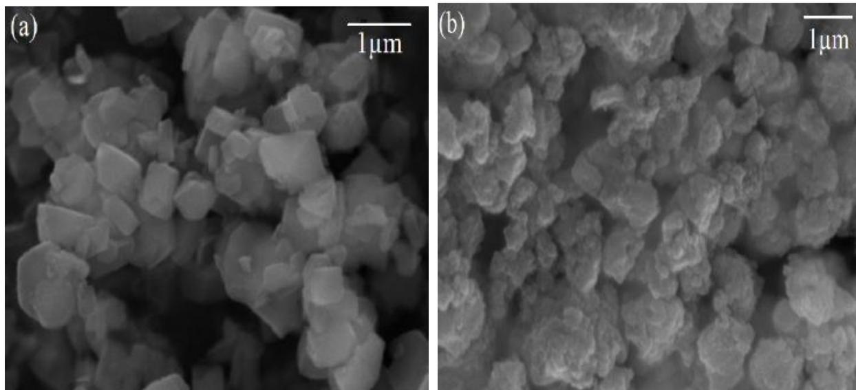
Figure 1 : (a) FE-SEM image of zeolite (b) SEM image of nZVI@zeolite particle
